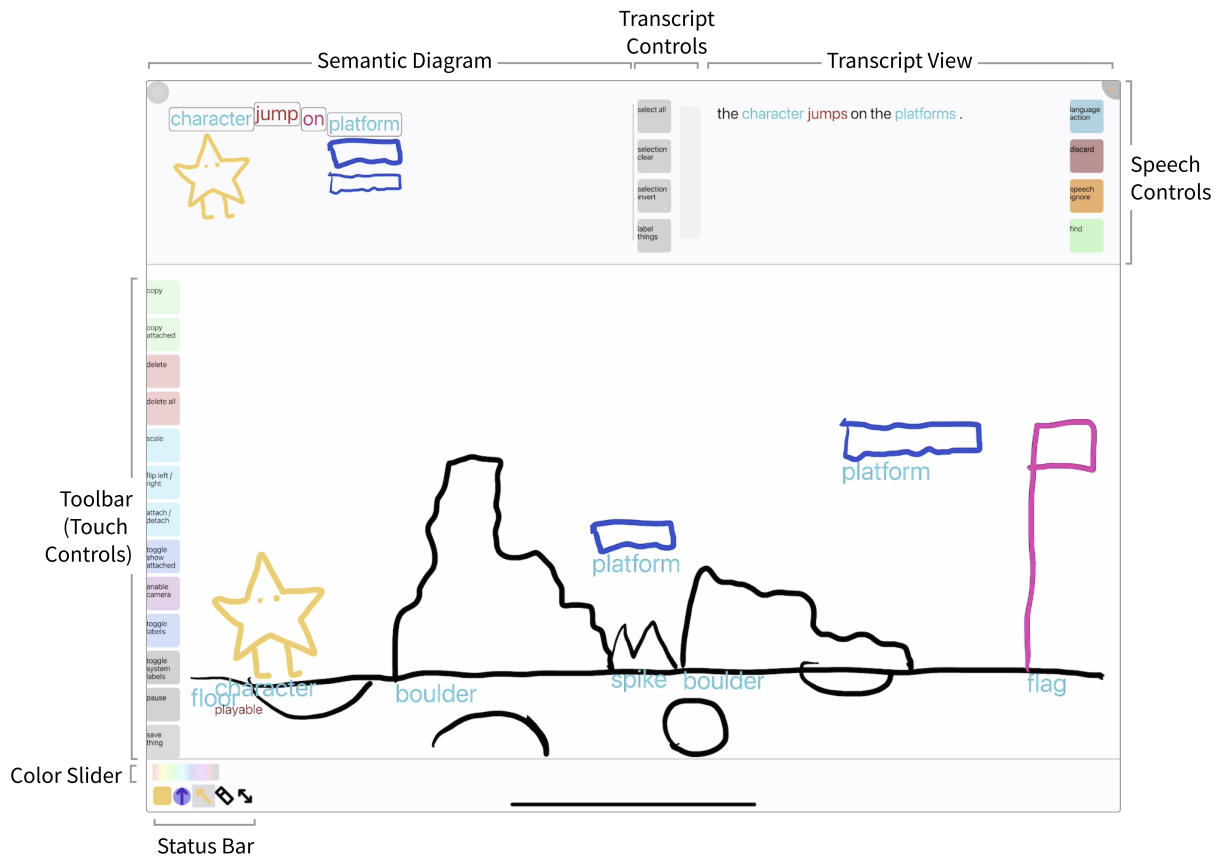
Figure 2: Interface Overview: An interface screenshot (from P4 in section 6). The toolbar (left) enables edit operations, e.g. copy, delete, attach/detach, save sketch. The transcript view displays the user’s speech input in an interactive panel, and the semantic diagram displays the machine’s understanding of the input. “Speech controls” stage/confirm an action, discard input, and toggle speech recognition. “Transcript controls” offer quick transcript text selection. The status bar displays the current color, a compass pointing “up,” and has the pen/eraser state-change buttons and indicators. The scene shown is just before the user confirms a command for the utterance “The character jumps on the platforms”; it selects the sketch labeled “character” and all sketches labeled “platform.” Tapping the “language action” button (top-right) will stage the command and display the semantic diagram (top-left) representing the machine’s understanding of the input with selected objects displayed under their respective words; the user confirms the command by tapping again. This causes the character to jump on all of the platforms. For details on the workflow and commands, see subsection 4.2 and subsection 4.4.
